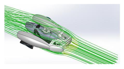
The **XLAB Torpedo Bottle** without any style of computer mount produces a drag savings of 56 grams / 5.6 watts compared to a rider without anything positioned between the arms.
