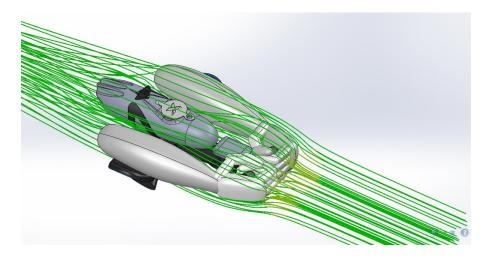
Using the XLAB Versa Computer Mount yielded zero change in drag compared to a XLAB Torpedo Bottle without any type of computer mount.
