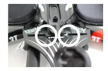
9. Secure the Velcro straps by routing them through the clamps. Pull the straps as tight as possible and attach them in place.
