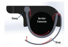
10. Tighten both mounting clamp screws and torque to 35 in lbs (4.0 Nm).
